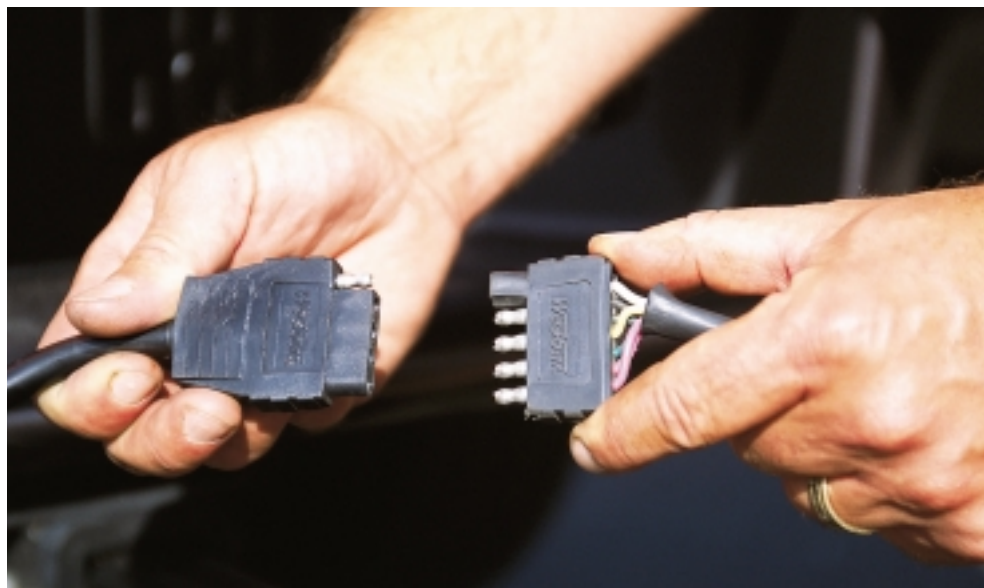
THIS FIVE-WAY PLUG USES a fifth circuit to lock out the trailer's disc brakes when you back up. An adapter may be needed to mate with the tow vehicle's plug.
