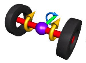
First, the differential. That's the purple sphere in the middle of the long axle housing that the wheels are connected to. If you poke your head under the rear of your 80, you'll see it (of course it's all painted black under there). Under the front of an 80, the diff is off to one side (RHS).
