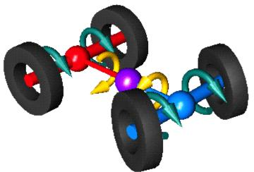
The centre diff (purple sphere) allows the front and rear drive shafts to turn at different rates whilst still driving both drive shafts.
