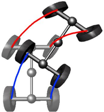
When we study the example on the left, we see that when turning a corner, the front wheels travel a longer distance (red curves) than the do the rears (blue curves).
