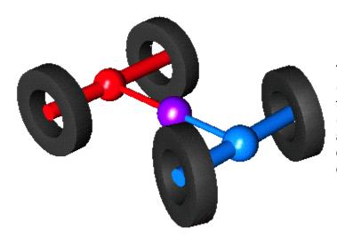
The 80 Series has 3 differentials (they're the 3 spheres shown to the left). One on the front axle (blue), one on the rear axle (red) and one in the transfer case (purple - referred to as the centre differential).
