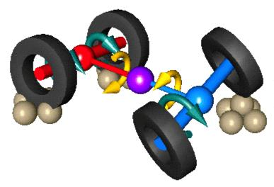
In our situation here, instead of all the drive being lost to the spinning wheel, with the centre diff locked, the rear drive shaft must now turn at the same rate as the front.
