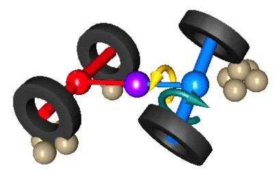
Right here, we're in a situation where we are climbing over uneven terrain and one wheel loses traction (the lower wheel on the blue axle).
