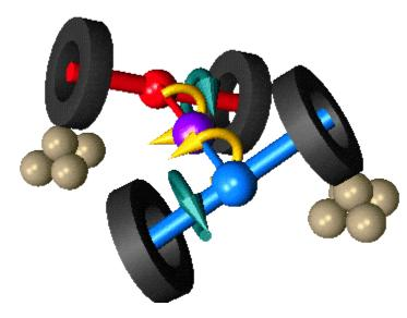
Now we're in a situation where a front and rear wheel has lost traction. Drive through the centre diff goes to the front and rear drive shafts and then to the wheels.
