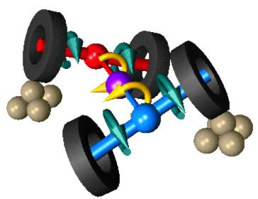
Taking this further, when the front diff lock is then locked, the left and right axles at the front are physically locked together and both front wheels must turn at the same rate.
