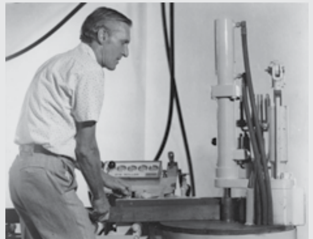
Reg Dobinson demonstrating his new invention, the 'Leaf Spring Eye Roller' 1977
