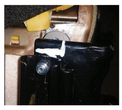
If your rail does **not** have a welded nut in this position then it will have a longer piece of metal at the back which requires some ginding.
