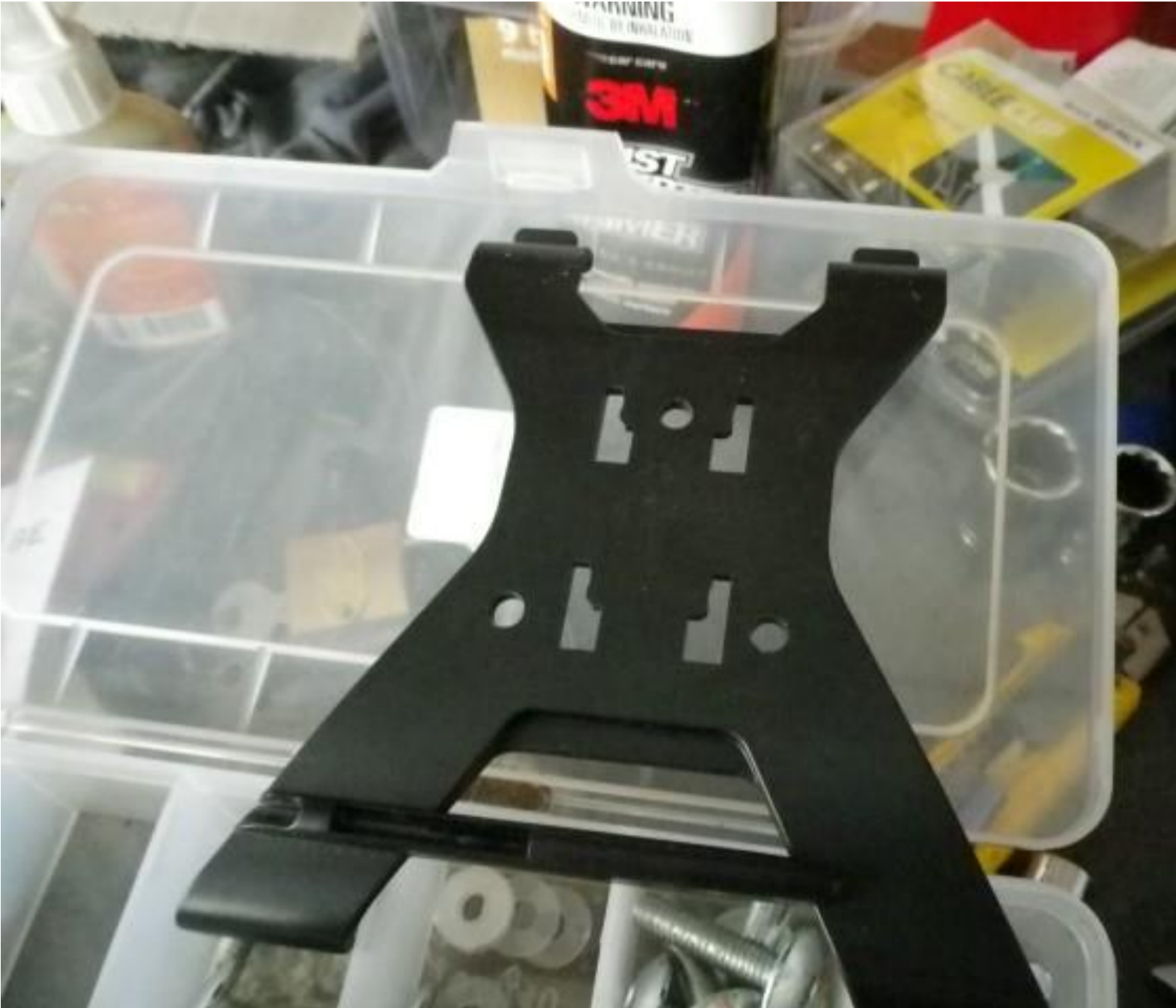
3 new holes in the VMS backing plate to match the Ram mou
