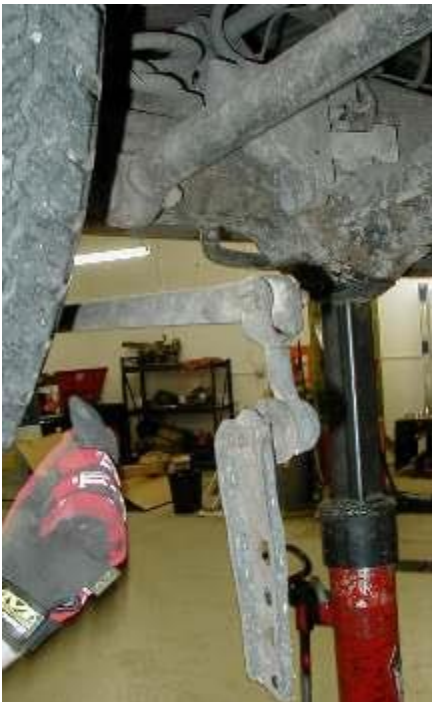
Rear swaybar disconnected
