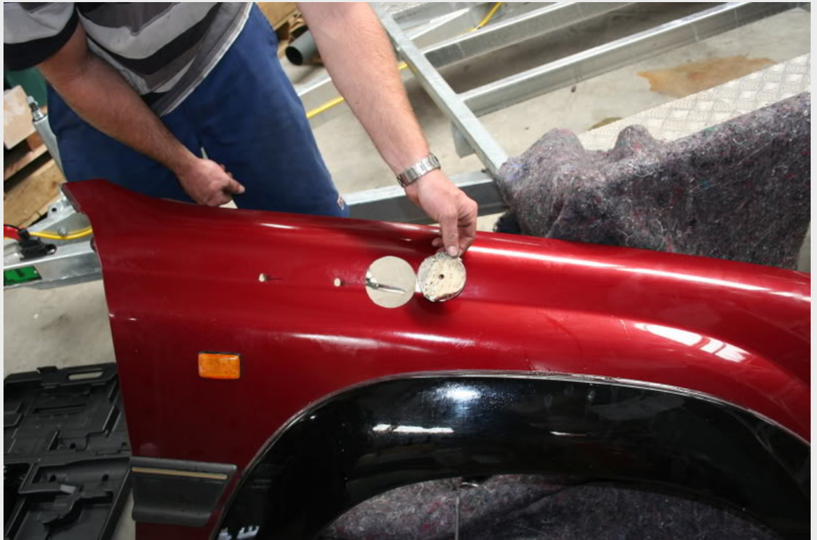
Do a test fit of the snorkle into the guard to check the holes line up. Mine did, but the snorkle wasn't sitting where it felt like it should to i slotted the mounting holes with the round file:
