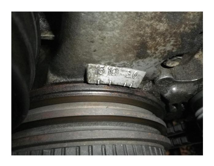
Timing is advanced/retarded by loosening this bolt slightly and moving the distributor(motor off) .. Mark its original placement so you can go back to where it was if necessary
