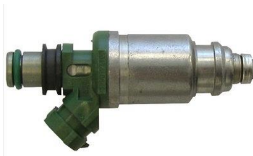
One of several different types of fuel injectors Toyota has used. This one fits 1997 to 2000 Camry & Celica.
